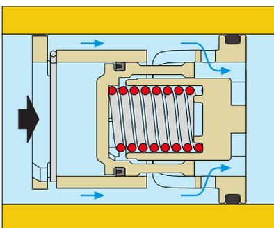
In this case, the piston fully compresses the spring and leaves only the fixed geometry aperture for the medium to pass through.
