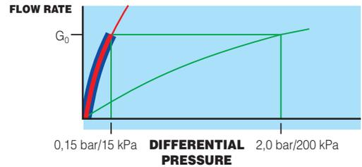
$$Kv_{0,01} = 0,258 \cdot G_0 \quad \text{range } \Delta p \text{ 15-200 kPa} \quad \text{where } G_0 = \text{nominal flow rate}$$
