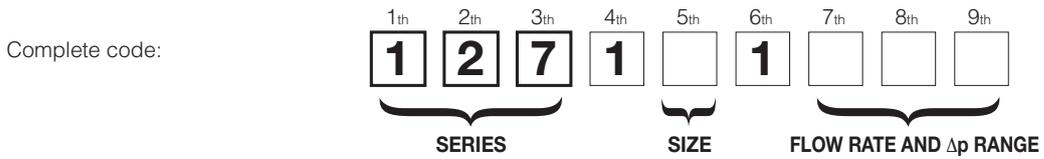
**SERIES**      1<sup>th</sup> 2<sup>th</sup> 3<sup>th</sup>      The first three digits indicate the series:      127 | AUTOFLOW® regulators
