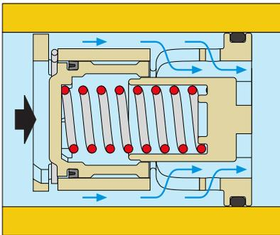
In this case, the regulating piston remains in equilibrium without compressing the spring and gives the fluid the maximum free flow area. In practice, the piston acts as a fixed regulator and thus the flow rate through the AUTOFLOW® depends solely on the differential pressure.
