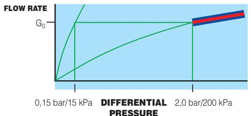
$$Kv_{0,01} = 0,070 \cdot G_0 \quad \text{range } \Delta p \text{ 15-200 kPa} \quad \text{where } G_0 = \text{nominal flow rate}$$
